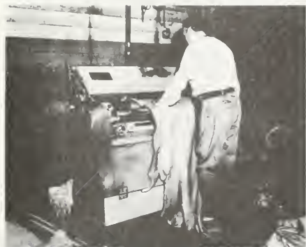
10. Shaving skins for additional thickness adjustment.
